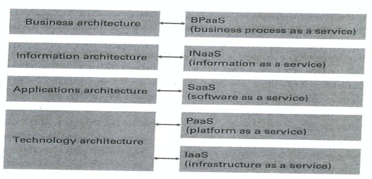
Figure 2 Enterprise architecture stack and cloud service models
