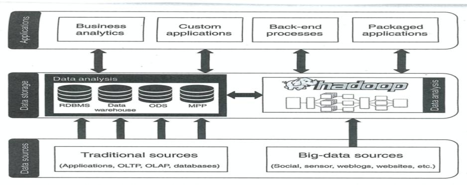
Figure 6 A typical small-data and big-data architecture for data science (inspired by a figure from the Hortonworks newsletter, April 23, 2013, https://hortonworks.com/blog/hadoop-and-the-data-warehouse-when-to-use-which).
